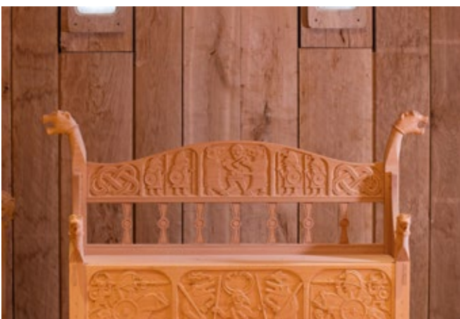
The decorations were created by the museum, based on original designs found in graves and excavations in Denmark, Sweden and Norway. Bystrup Maskinsnedkeri received them as STEP files, which were imported into ALPHACAM. The designs sank into the wood to a depth of 25mm, and were machined with small ball nose cutters, which were required to achieve the necessary detail.
